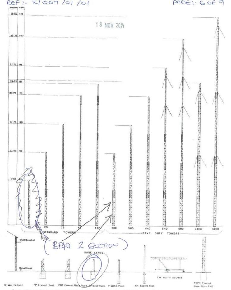
To specify a particular tower merely quote the tower/ base; e.g. a 35/FP is a standard 35 tower complete with FP type base.
