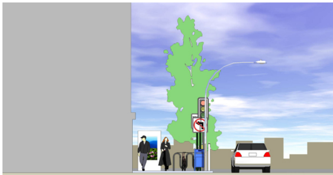
Figure 5.10 Street Clutter obscures views along the street and can cause obstructions for pedestrians
