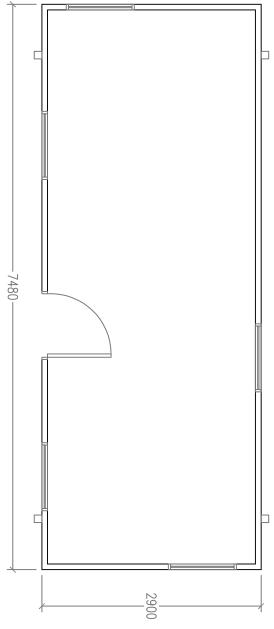
The proposed portable office accommodation will have a flat roof constructed from plastic coated steel sheet in a light grey colour. The walls of the office will be plastic coated flat steel sheet in a light grey colour. The door will be a steel door in a light grey colour. Windows will be double glazed uPVC in a white colour.
