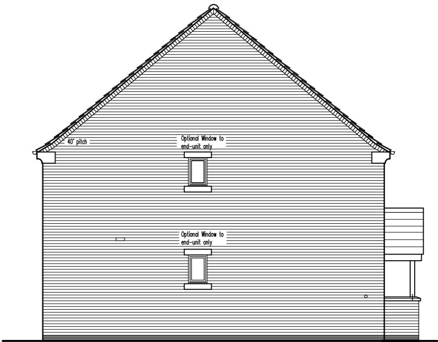
SIDE ELEVATION INDICATING OPTIONAL WINDOWS TO SIDE ELEVATION
