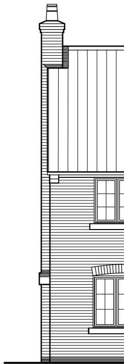
FRONT ELEVATION INDICATING OPTIONAL PROJECTING CHIMNEY
