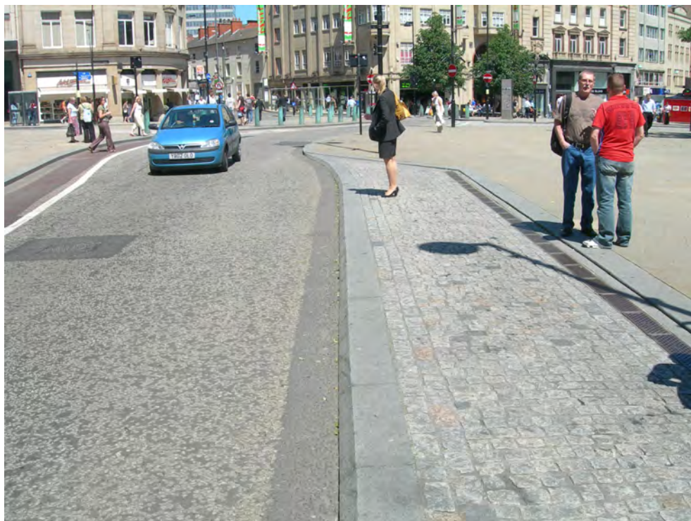
Figure 4.17 The provision of modest elements such as lay-by service areas can be enhanced and distinguished by use of contrasting and high quality paving material (Sheffield City Centre)
