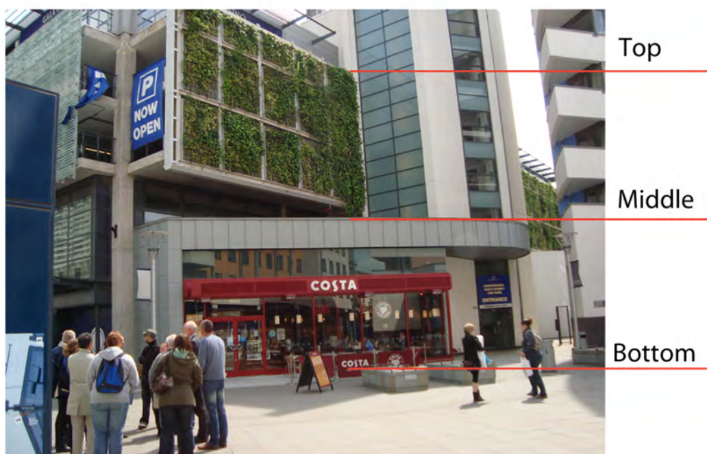
Figure 4.4 Example of a frontage which is made active at ground floor level by its use as a coffee shop. The middle section of the façade is an inactive green wall with the top of the façade recessed above (Bristol City Centre)
