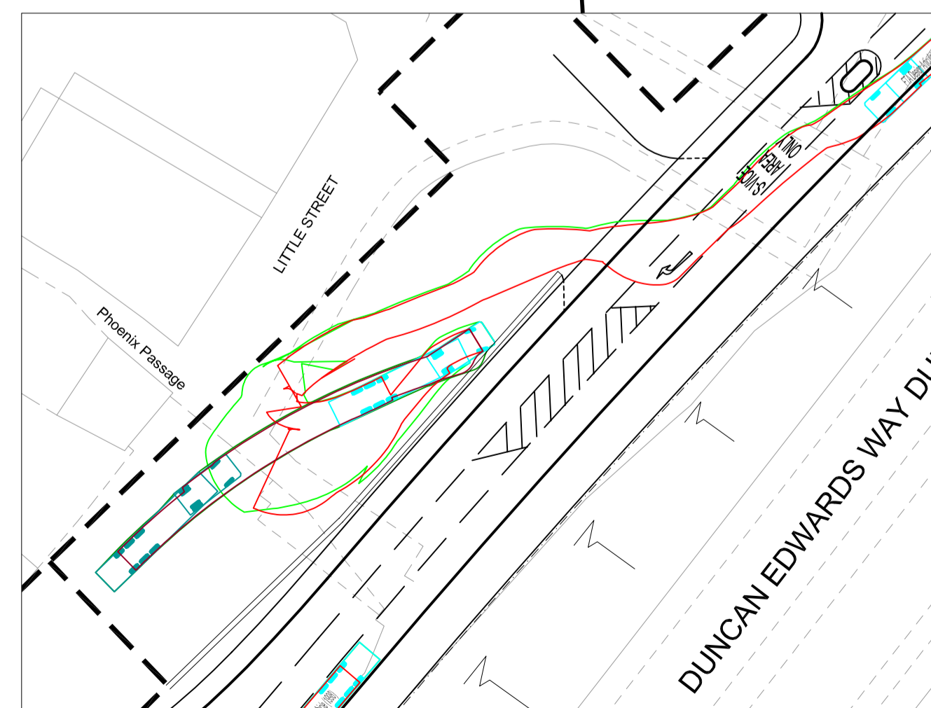
South Service Yard Access Scale 1:500
