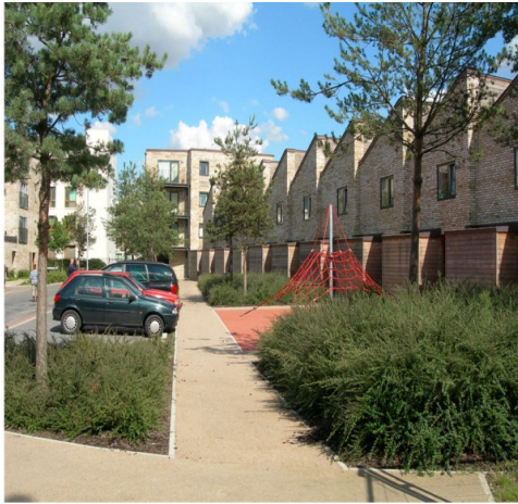
Left, trees and soft landscaping no higher than 600mm are used to soften the visual impact of parking, right, breaks in parking bays
