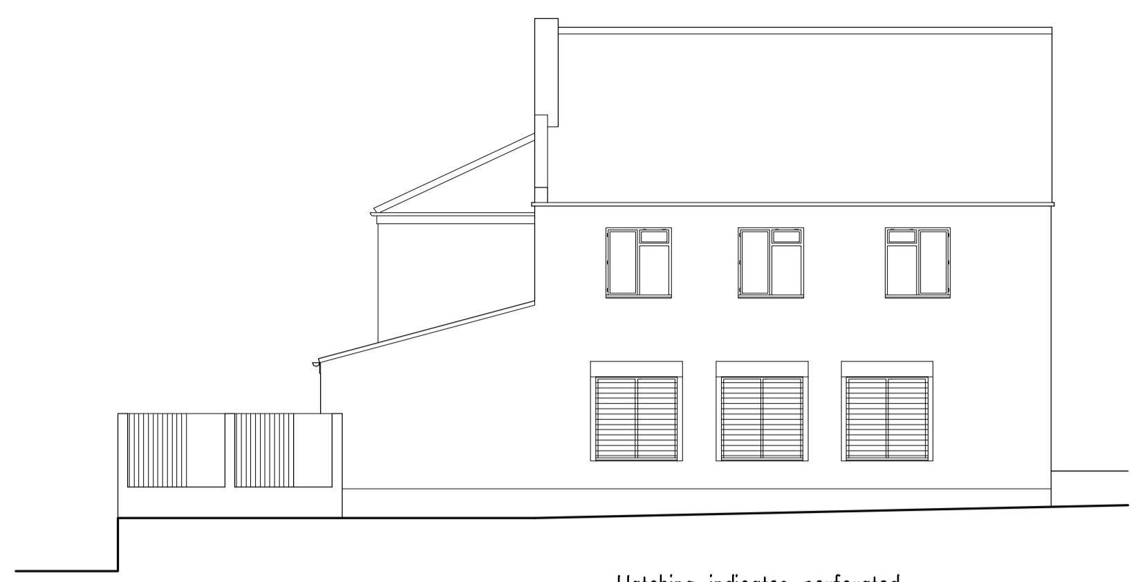
Front elevation Hatching indicates perforated security shutters
