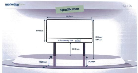
Signs mounted on 1000mm x 50mm black posts. Non-Illuminated / Non-Reflective signage. (Matt finish) Signs will be positioned a minimum of 1000mm away from the roundabout edge.
